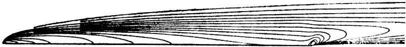
FIG. 155.—VORTICITY CONTOURS TO OSEEN'S APPROXIMATION FOR A FLAT PLATE AT R = 4 \times 10^4 .
