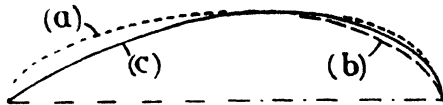
FIG. 90.—THICKNESS DISTRIBUTION OF SYMMETRICAL AEROFOILS WITH MAXIMUM THICKNESS AT 0·4 CHORD FROM NOSE.
